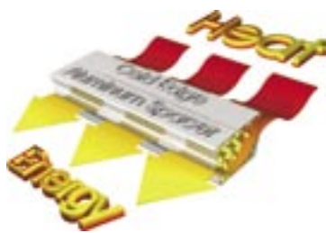
Insulating glass spacers constructed of aluminum and steel conduct heat energy.
